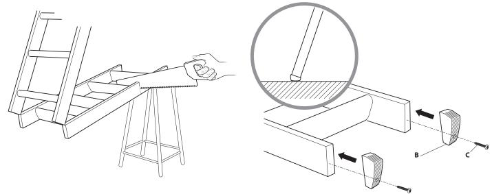
Saw off the excess piece of the ladder on both sides.
