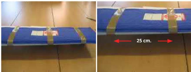
Make sure the thermostat (red circle on the label) is in contact with the surface. The best way is with tape or straps as shown.
