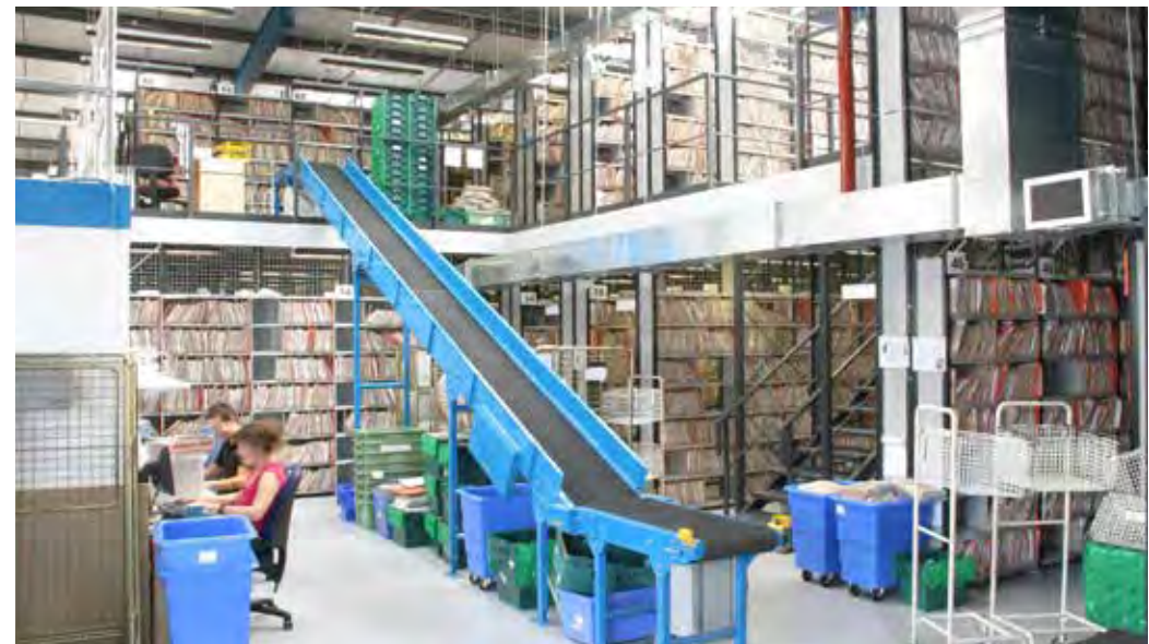
Two tier shelving is widely used for document archiving and is a cost-effective solution for utilising the height available. The ground floor shelving provides the structure to support the raised walkways.
