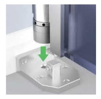
**STEP 2** After placing the washer mount the door onto the base plate.
