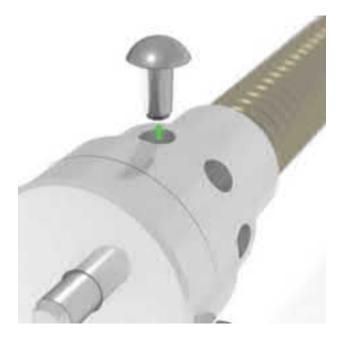
**STEP 2** Remove the tensioning pin from existing hole location.
