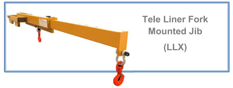
Tele-Liner jib offers a solutuion to the hadling of previously inaccessible loads. To fit; simply remove the attachment heel pin and drive the truck slowly forwards until the forks are fully sleeved. Then simply re-fit the heel pin behind the forks of the truck. Ensure the jib is fully secured before lifting commences.
