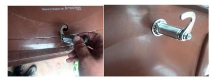
3 Remove nut and washer, insert lock and arm through hole. Replace washers and nut, tighten with shifting spanner or similar.
