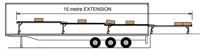
This heavy duty expressway offers an additional model allowing an extended length of 15meters. All decks are reinforced with rolled steel angle and include a strengthened transfer and pivot area.
