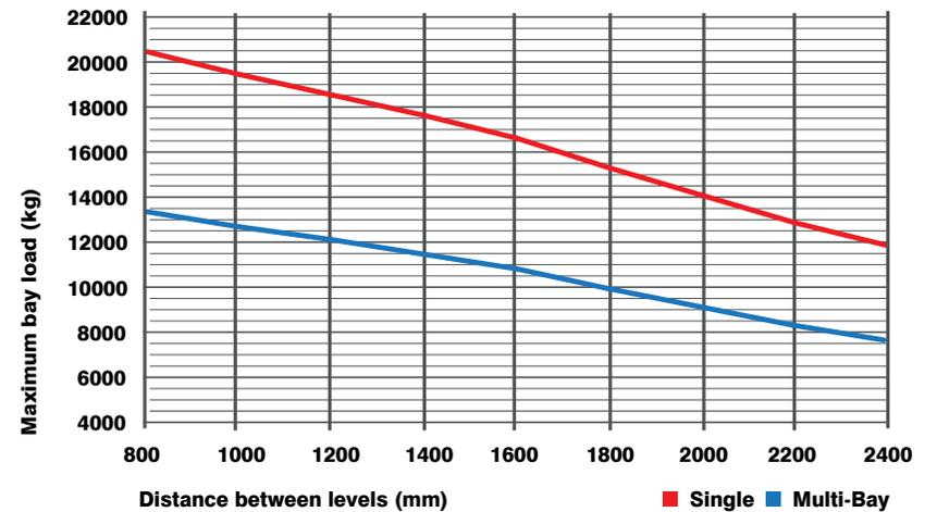
Frame capacity is calculated at a beam pitch of 1500mm, and a run of five 2700mm wide bays
