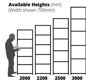
Price includes 4x uprights, 6x shelves and all necessary fixings, bracing and plastic feet. Extension bay comes with 2 uprights only. 1 pair of Cross Bracing required per four bays.
