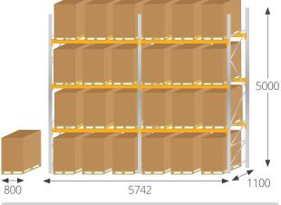
• Pallet Racking Kit 6 for 24 x pallets (Boxes shown H: 1200 x W: 800mm)
