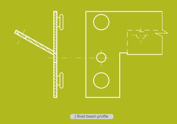
J Rivet increases storage density with its 30mm slim beam profile.
