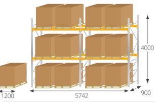
• Pallet Racking Kit 2 for 12 x pallets (Boxes shown H: 1500 x W: 1200mm)
