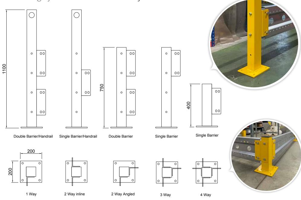
(i) Our moulded rack protectors offer a high visibility bumper, which suits many of the leading pallet racking systems. Available from - Merlin Industrial Products Ltd - 0800 0418 650 - info@merlin-industrial.co.uk
