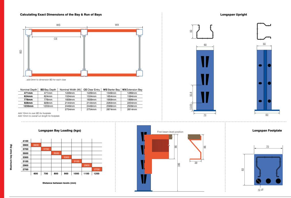
(i) Remember, if your shelving's height to depth ratio is greater than 4:1, the bay should be fixed to the floor or to the wall! Available from - Merlin Industrial Products Ltd - 0800 0418 650 - info@merlin-industrial.co.uk
