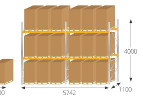
• Pallet Racking Kit 5 for 18 x pallets (Boxes shown H: 1500 x W: 800mm)
