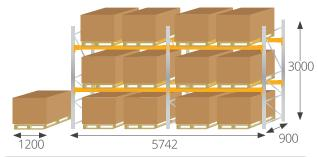
• Pallet Racking Kit 1 for 12 x pallets (Boxes shown H: 1000 x W: 1200mm)
